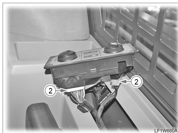
13. Disconnect the A/C controller wiring connector (2).
