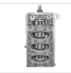
4. Unscrew the main bearing bolts (1) (10 EA) from the bottom of the cylinder block.
