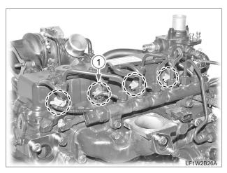
10. Disconnect injector solenoid connector (1).
