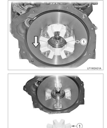
52. Remove the coupling element (1) from the flywheel.
