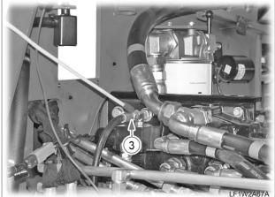
17. Install the return hose (3) between the main control valve and the oil tank.
