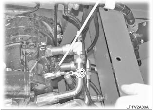
24. Install the return hose (10) between the HST motor (LH) and the oil tank.
