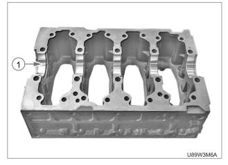
4. Install the crankshaft bearing (lower) (1) to the ladder frame..
