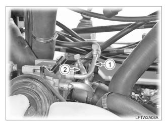
34. Disconnect the A/C hoses (1: high-pressure, 2: low-pressure) from the compressor.
