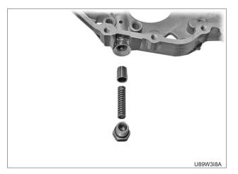
14. If necessary, remove the relief valve.
