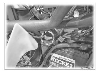
Open the rear cover and disconnect the negative (-) battery cable.
