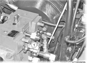
15. Connect the return hose (1) from the HST pump to the oil tank.
