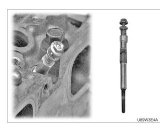
1. Screw out the glow plug (1) from the intake side of the cylinder head.
