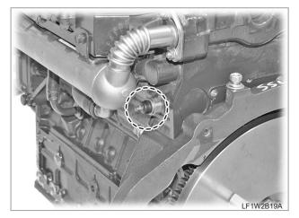
• Engine oil pressure sensor
