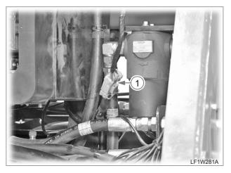
17. Disconnect the wiring connector (1).
