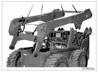
Support the boom with a hoist. Then, remove the lift cylinder retaining pins (1), boom auxiliary support pins (2) and boom retaining pins (3) to remove the boom assembly (4).
