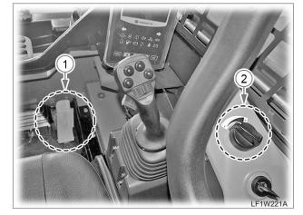
When depressing the accelerator pedal (1) or moving the engine throttle dial (2) to select a high speed, detects the amount of movement of the acceleration position sensor and sends this information to the ECU which then permits combustion in the chamber to increase the engine RPM and power.
