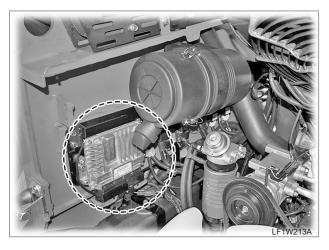
The ECU (Electronic Control Unit) is the most important information processor in the engine as it analyzes information sent from various sensors and takes an appropriate action for optimum engine performance.
