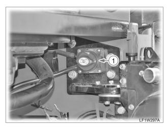
28. Remove the battery power cut-off switch (1).
