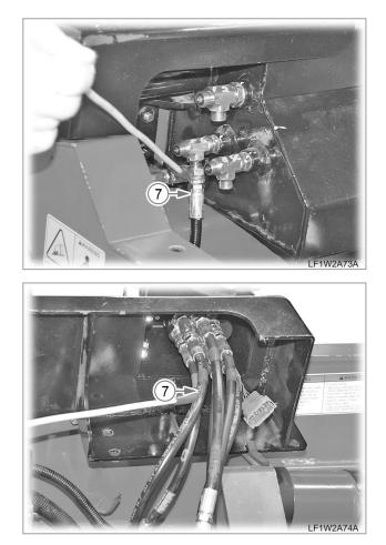
21. Install the left-hand RCV assembly return hose(7) on the oil tank.
