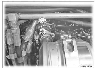
After disconnecting the CCRT wiring connector and connecting rod (1), unscrew the CCRT mounting bolts (2) and nuts (3) to remove the CCRT assembly (4).
