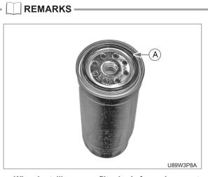
• When installing a new filter body for replacement, apply a thin film of oil onto the O-ring surface (A) and tighten the filter firmly with a hand.
