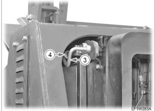
18. Install a refrigerant collector to the A/C hoses (1 & 2) and collect the refrigerant. Then, disconnect the A/C hoses (3 & 4).
