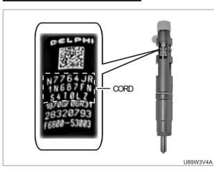
The code C3I is marked on the side of the injector and cylinder head cover. This code consists of 20 digits including numbers from 1 to 9 and alphabetic characters excluding I, O, Q and V.
