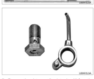
7. Remove the piston cooling jet valve (1) from the cylinder block as necessary.
