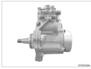
3. Unscrew the high-pressure fuel pump mounting bolts (3) to remove the high-pressure fuel pump assembly.
