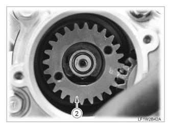
2. Remove the high-pressure fuel pump gear (2) from the gear case.
