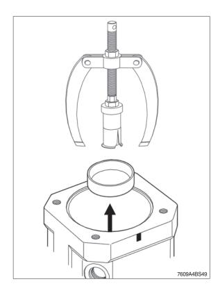
(13) Disassemble circlip and shaft seal.
