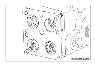
Fit stop for priority valve spool (thickness : 8 mm) with vaseline.
