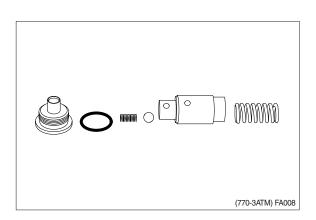
⑦ Counter pressure valve with orifice shown disassembled.
