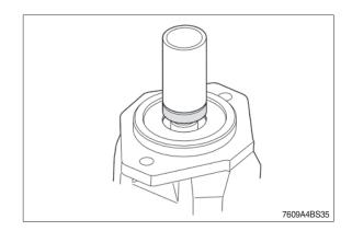
(6) Assemble the circlip.
