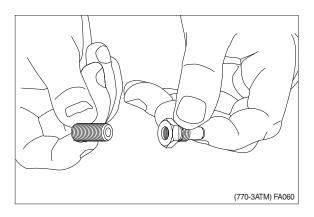
Shock valve / suction valve shown disassembled.
