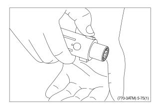
(13) Remove dust seal and O-ring.
