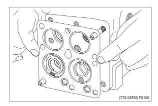
7 Fit stop (thickness: 5 mm) in end cover with vaseline.
