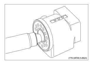
(17) Press and turn the lip seal into place in the housing.
