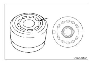
(5) Mounting surface - control plate undamaged.
