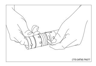
⑥ Push spring ring into position. Place spring ring into the recess with ends facing away from pin holes.
