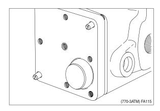
$\ensuremath{{\mbox{\scriptsize{}}}}$  Fit large screw with spring washer.
