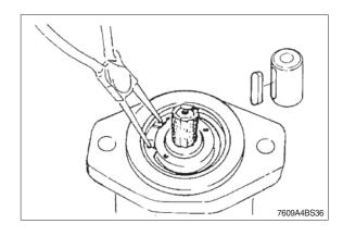
(7) Assemble the circlip in the correct position.
