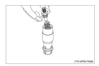
⑤ Tighten with torque wrench for 19 mm external hexagon. Use a mandrel.
