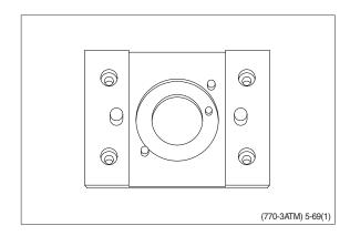
(2) Assembly tool for O-ring and kin-ring.
