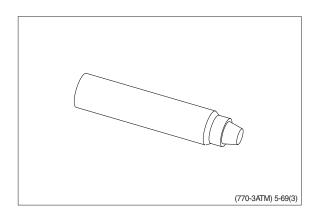
(4) Assembly tool for cardan shaft.
