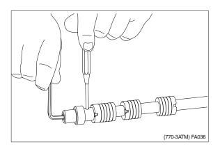
② Directional spool shown disassembled.
