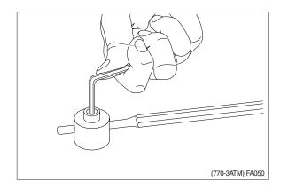
① Amplifier spool shown disassembled.
