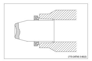
(16) Guide the assembly tool right to the bottom.
