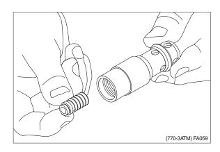
① Unscrew adjustment screw and take out spring and ball.
