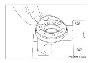
(23) Place the distributor plate so that the channel holes match the holes in the housing.
