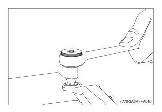
② Screw pressure relief valve out (10 mm hexagon key).
