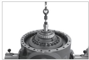
4 Insert the determined shim (e.g. s = 1.4 mm) into the bearing housing and reset the bearing outer ring until contact is obtained.
