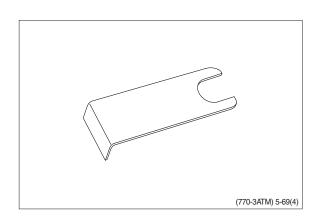
(5) Assembly tool for dust seal.
