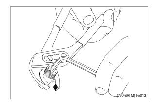
② Pressure relief valve shown disassembled.
