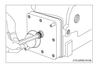
10 Fit screws with spring washer.
