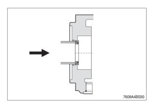
(14) Remove shaft seal and shim.
