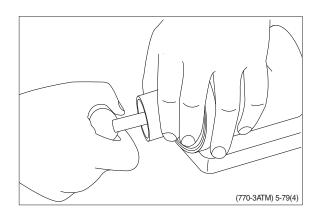
(14) Draw the inner and outer parts of the assembly tool out of the steering unit bore, leaving the guide from the inner part in the bore.
