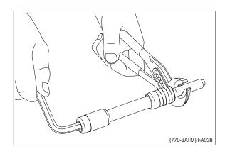
② Priority valve spool with plug for external PP shown disassembled.
