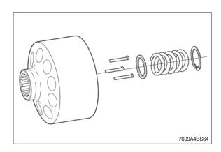
(7) Pre-tension the spring using a suitable device.
