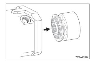
(8) Remove the drive shaft to rear side.
