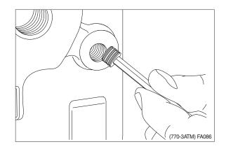
③ Fit throttle check valve in PP connection.
