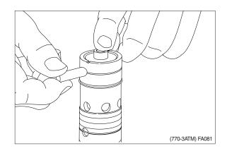
① Push spring ring into position. Place spring ring into the recess with ends facing away from pin holes.
