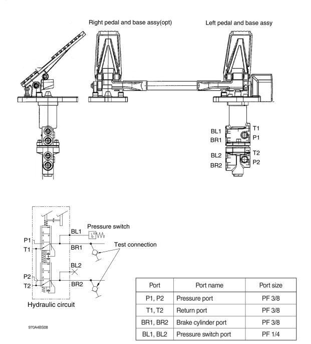
· Brake pressure specification :  $80\pm5$  bar ( $1160\pm70$  psi)
