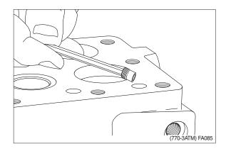
② Fit orifice in LS - connection.
