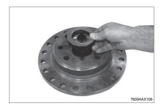
I Mount two adjusting screws and insert the housing cover until contact with the differential housing is obtained.
