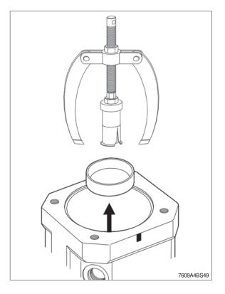
(13) Disassemble circlip and shaft seal.
