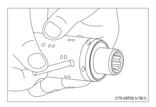
(9) Fit bearing races and needle bearing as shown on below drawing.
