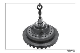
⑤ Preload the compression spring by means of the press and disengage the retaining ring.
