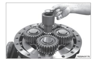
③ Fix O-ring (see arrow) with grease into the countersink of the brake housing.
