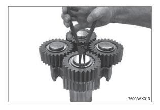
13 Pull off planetary gear.
