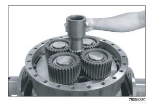
25 Fix determined shim e.g. s = 1.00 mm with grease into the sun gear shaft.
