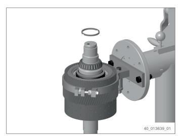
Insert bearing outer rings into helical gear until contact is obtained.
