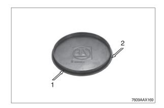
(25) Insert the cover into the output shaft until contact is obtained.
