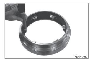
Insert the piston into the brake housing and carefully install with the fixing device until contact is obtained.
