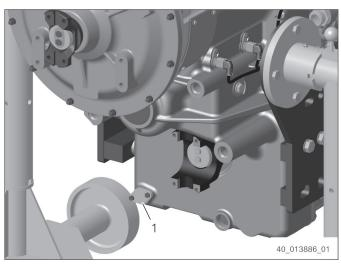
2. Loosen hexagon screws and remove cover sheet with seal (1).
