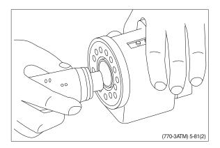
(19) The spool set will push out the assembly tool guide. The O-ring are now in position.
