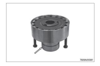
(6) Position the premounted differential with the lifting device onto the housing cover and preliminarily fix with hexagon screws.
