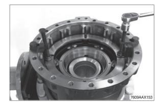
Insert disk and cup spring with the convex side showing upwards into the piston.
