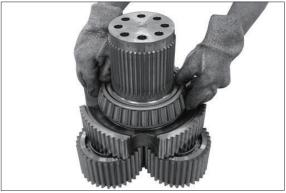
Wet front face (contact face bearing inner ring, arrow 1) and profile (teeth, arrow 1) in the output shaft with anticorrosive agent.
