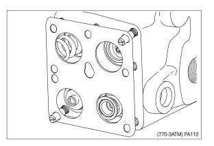
④ Fit stop for priority valve spool (thickness : 8 mm) with vaseline.
