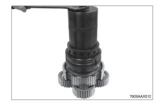
12 Disengage retaining ring.
