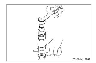
① Unscrew orifice out of plug with 4 mm hexagon key. Use a mandrel.
