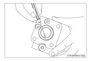
(14) The steering unit is now completely disassembled.
