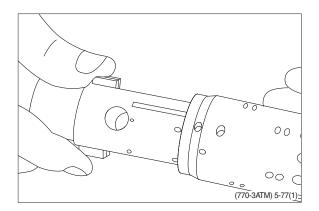
(5) Press the springs together and push the neutral position springs into place in the sleeve.
