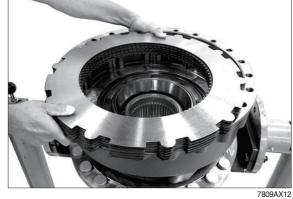
15 Loosen hexagon screws, remove releasing disk and cup spring.
