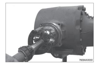
(5) Loosen slotted nut and remove the shim behind.
