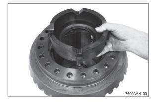
(5) Insert the axle bevel gear until contact is obtained and install the inner disks with the teeth.
