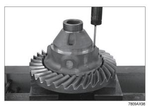
① Pull spider shafts (4EA) and remove the releasing spider gears with the thrust washers from the differential housing.
