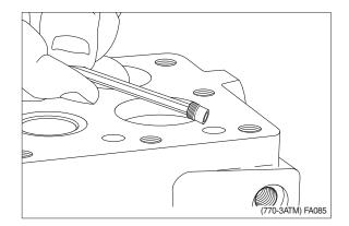
2 Fit orifice in LS - connection.
