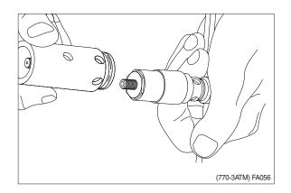
④ Unscrew pilot valve with hexagon socket for 19 mm external hexagon. Use a mandrel.
