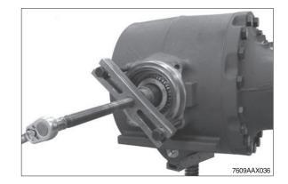
8 Remove spacer ring and pull the tapered roller bearing from the input pinion.
