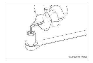
(2) Check valve shown disassembled.
