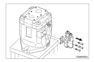
(2) Measure dimension A and note down.Check sealing surface (1).Replace gasket (2).
