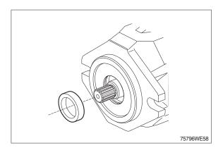
(3) Assemble the sealing ring, fitting tool holds the correct position of the sealing ring in the pump housing. Assemble the circlip in the correct position.
