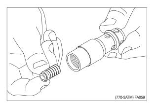
⑦ Unscrew adjustment screw and take out spring and ball.
