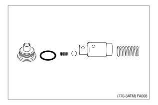
⑦ Counter pressure valve with orifice shown disassembled.
