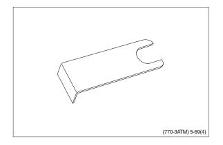
(5) Assembly tool for dust seal.
