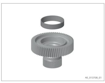
63. Slide spur gear (1) onto shaft until contact is obtained. Insert spur gear into disk package by short mutual rotary motions.
