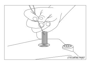
6 Counter pressure valve shown disassembled.
