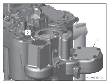
Pull pin (1) with AA02.242.247 [Extracting device] and AA02.571.771 [Adapter] out of the housing hole. Remove gear (2), bearing inner rings and shim.
