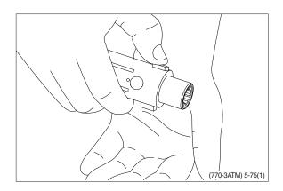
(13) Remove dust seal and O-ring.
