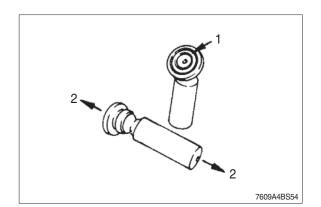
(2) Check cylinder bores (1) and splines (2).
