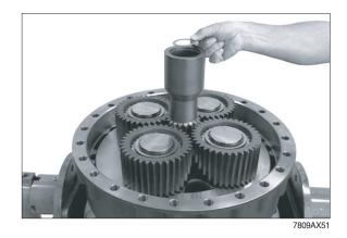
② Fix O-ring (see arrow) with grease into the countersink of the brake housing.
