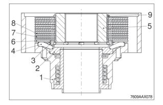
(3) Preload disk package with an axial force of  $F = 50^{+30}$  kN.
