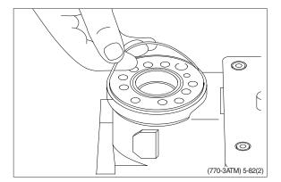
(23) Place the distributor plate so that the channel holes match the holes in the housing.
