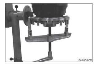
① Lift the planetary carrier out of the brake housing by means of the lifting device.
