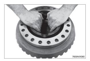
⑦ Press crown wheel from the differential carrier.
