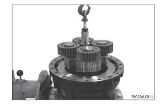
Pull the tapered roller bearing from the planetary carrier.
