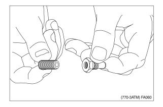
⑧ Shock valve / suction valve shown disassembled.
