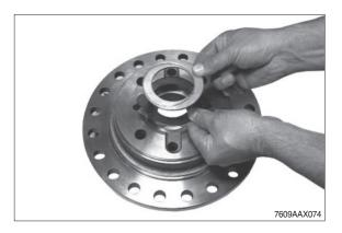
In Mount two adjusting screws and insert the housing cover until contact with the differential housing is obtained.
