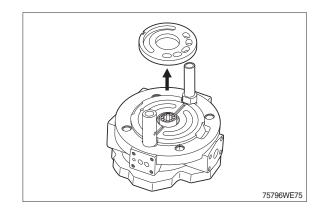
(12) Use bearing puller to remove outer bearing race of rear bearing - press seat.
