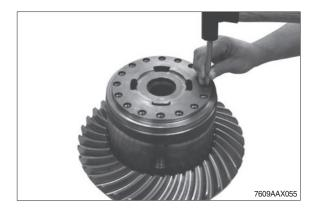
6 Force out both differential axles (short) and remove the releasing spider gears with thrust washers from the differential housing.
