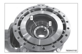
(9) Align disk package centrally and radially.
