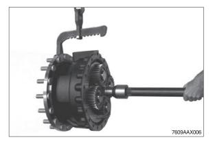
6 Fix output to assembly truck.
