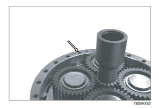
⑦ Grease O-ring (see arrow) and install it to the axle housing.
