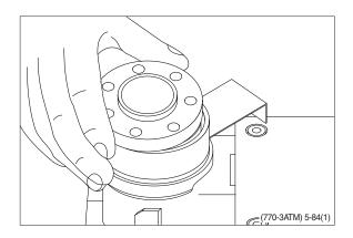
(30) Fit the special screw with washer and place it in the hole shown.
