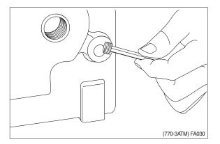
② Unscrew throttle check valve in PP-connection with 6mm hexagon key.
