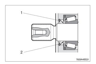
(2) Remove key.Protect the drive shaft.Remove the circlip.
