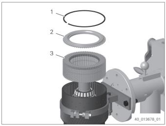
Pull off bearing inner ring with 5873.001.034 [Gripping device] and 5873.001.000 [Basic tool].
