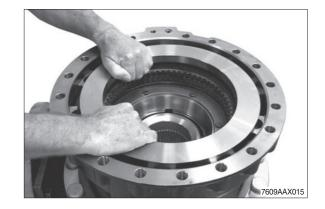
Is Lift the disk package out of the brake housing.
