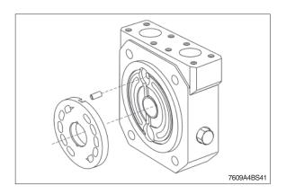
(5) Remove bearing outer ring with withdrawal tool.Do not damage the sealing surface.
