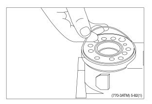
(22) Grease the O-ring with mineral oil approx. viscosity 500 cSt at 20 $_{\circ}\,$  C .
