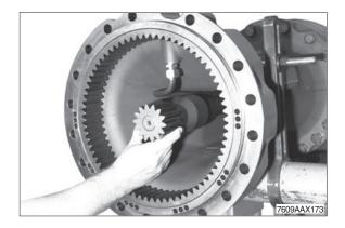
② Measure dimension II, from the front face of the sun gear shaft to the mounting surface of the axle housing.
