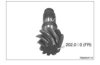
③ Determine dimension III (bearing width).
