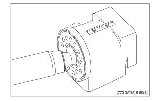
(17) Press and turn the lip seal into place in the housing.
