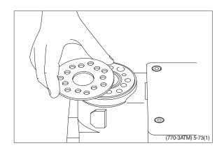
(6) Screw out the threaded bush over the check valve.
