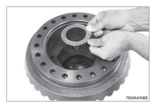
3 Insert axle bevel gear.
