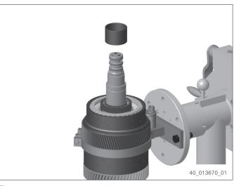
66. Insert snap ring into annular groove of the gear.
