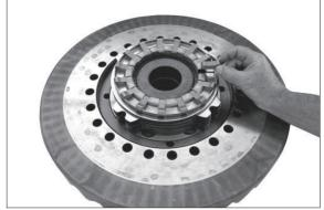
(5) Insert pressure piece (see arrow) and install disk.
