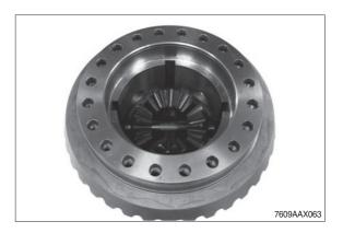
5 Remove the second axle bevel gear.
