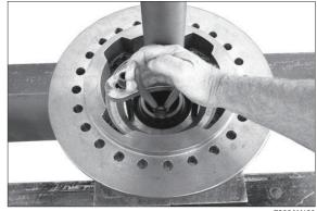
(9) Mount two adjusting screws and insert the differential cover by means of the lifting device.
