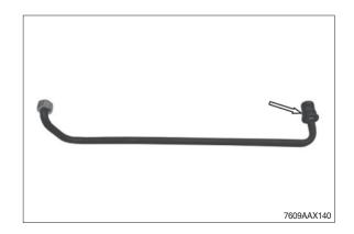
(5) Mount brake tube with threaded connection and hexagon nut (see arrow).
