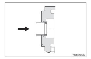
(14) Remove shaft seal and shim.
