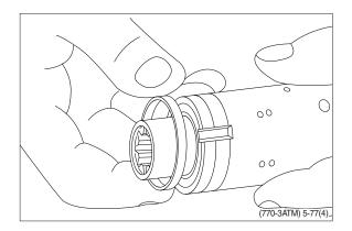
(8) Fit the cross pin into the spool / sleeve.
