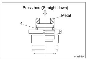
④ Fit rod seal (6), back up ring (7) and buffer seal (8) to corresponding grooves,
