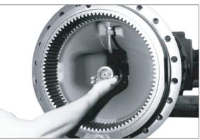
2 Insert the sun gear shaft until contact is obtained.
