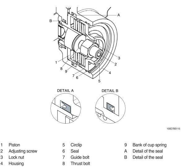
\* Faulty seals must be exchanged in accordance with the instructions below.
