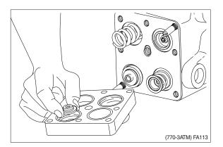
(5) Fit stop for directional spool (thickness : 5 mm) with vaseline.
