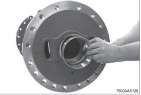
(9) Mount two locating pins and bring the axle housing into contact position with the axle drive housing by means of the lifting device.
