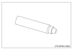
(4) Assembly tool for cardan shaft.
