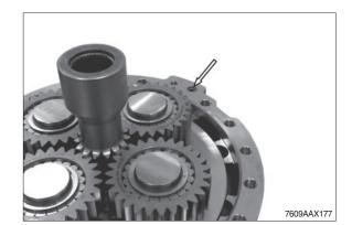
③ Grease O-ring (see arrow) and install it to the axle housing.
