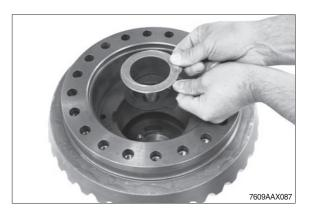
3 Insert axle bevel gear.
