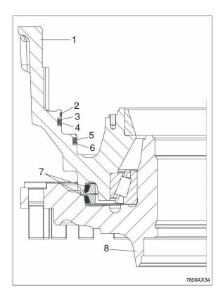
⑥ Insert the piston into the brake housing and carefully install with the fixing device until contact is obtained.
