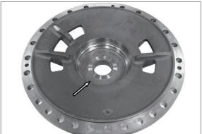
Determination of shims for setting of bearing rolling torque (differential housing) and backlash (bevel gear set)
