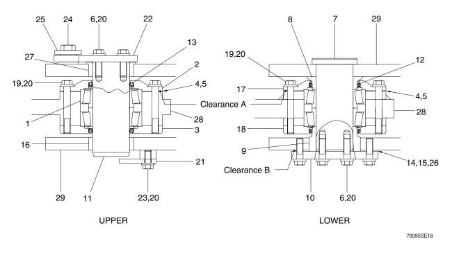
Assemble the center pivot group by reversing the order of disassembly while paying close attention to the following.
