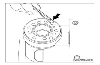
(21) Screw the threaded bush lightly into the check valve bore. The top of the bush must lie just below the surface of the housing.
