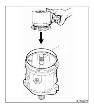
(7) Fit bearing (1) in connection plate.Fit cyilindrical pin (2).Fit O-rings (3) 4 pieces.Fit adjustment spool (4) and guide piston (4a).
