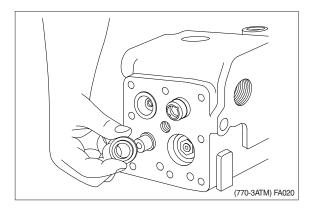
(5) Removing end cover at LS-connection
