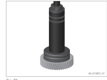
9. Use protective chucks made from aluminum.
