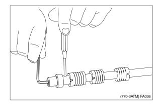
② Directional spool shown disassembled.
