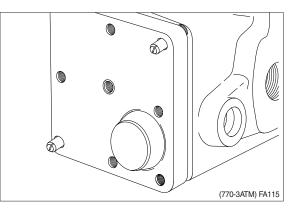
$\bigcirc$  Fit large screw with spring washer.
