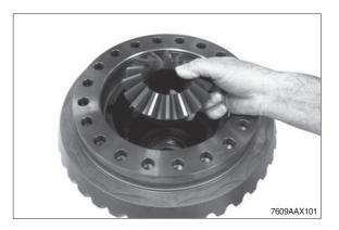
⑥ Preassemble the differential spider and insert it into the differential housing/into the pressure ring.
