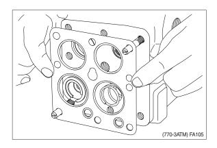
$\textcircled{\sc 0}$  Fit stop (thickness : 5 mm) in end cover with vaseline.
