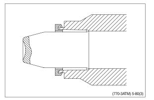
(16) Guide the assembly tool right to the bottom.
