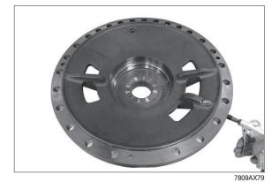
6 Lift differential out of the axle drive housing with the lifting device.
