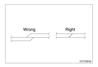
\* Back up ring (7) has its own fitting direction.
