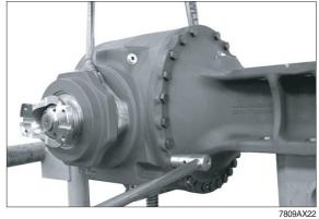
② Fix axle drive housing to the assembly truck.
