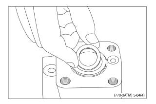
(33) Fit the dust seal ring in the housing.
