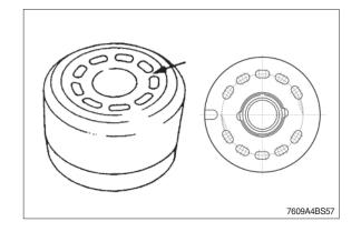
(5) Mounting surface - control plate undamaged.
