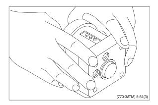
(20) Turn the steering unit until the bore is vertical again. Put the check valve ball into the hole indicated by the arrow.
