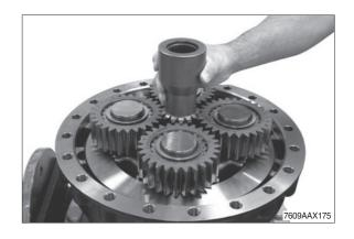
(1) Fix determined shim (s) e.g. s = 1.60 mm with grease into the sun gear shaft.
