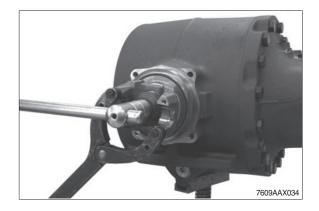
⑥ Pull the input flange from the input pinion and use a lever to remove the shaft seal behind from the axle drive housing.
