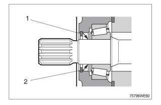
(2) Change the shaft seal and check its sliding surface (drive shaft) and housing, grease the sealing ring.
