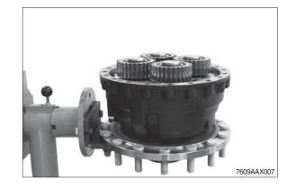
⑦ Use a lever to remove the cover from the output shaft.
