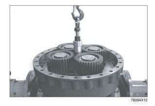
Description Pull the tapered roller bearing from the planetary carrier.
