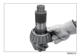
Setting of rolling torque of input pinion bearing 0.1~0.5 kgf·m (without shaft seal ring)
