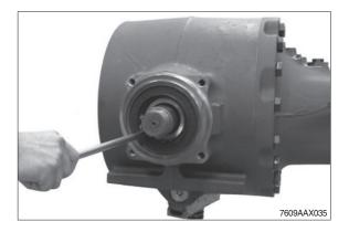
⑦ Press input pinion from the axle drive housing and remove the releasing tapered roller bearing.
