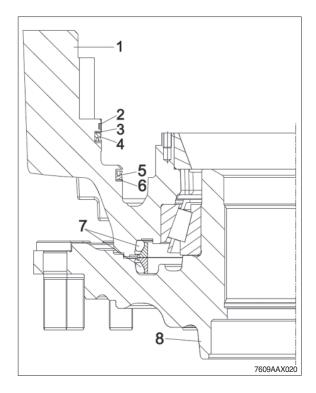
③ Lift the brake housing from the output shaft by means of the lifting device.
