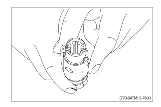
(4) Guide the spool into the sleeve. Make sure that spool and sleeve are placed correctly in relation to each other(See page 3-76, No.(1)).
