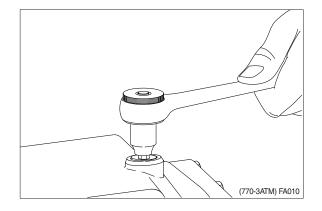
② Screw pressure relief valve out (10 mm hexagon key).
