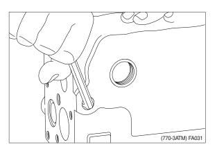
③ Unscrew orifice in housing with 4 mm hexagon key.
