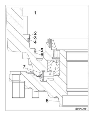
8 Flush-mount the slotted pins (6EA) into the holes of the piston.
