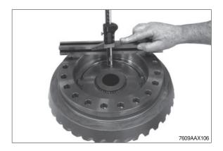
Measure dimension II, from the contact face of the outer disk to the mounting face on the housing cover.
