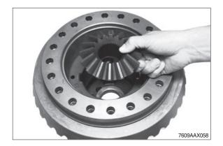
9 Press crown wheel from the differential carrier.
