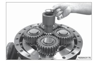
③ Fix O-ring (see arrow) with grease into the countersink of the brake housing.
