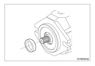
(3) Assemble the sealing ring, fitting tool holds the correct position of the sealing ring in the pump housing.Assemble the circlip in the correct
