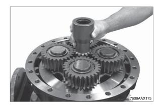
(i) Fix determined shim (s) e.g. s = 1.60 mm with grease into the sun gear shaft.
