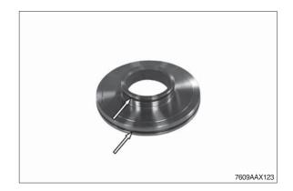
Insert piston (see arrow) into the bearing housing until contact is obtained.
