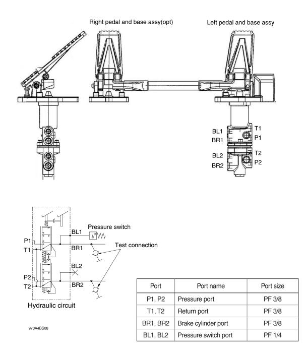
$\cdot$  Brake pressure specification : 80  $\pm$  5 bar (1160  $\pm$  70 psi)
