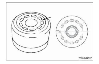
(5) Mounting surface - control plate undamaged.
