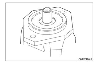
(5) Use a suitable pipe to mount the shaft seal, but don't push it too deep. If the shaft ring touches the bearing ring you will damage the seal ring.
