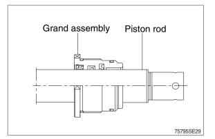
4 Fit piston assembly to piston rod.
