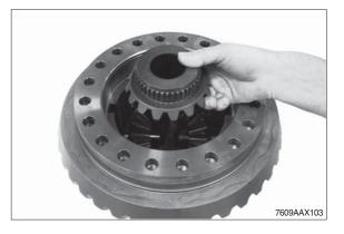
⑧ Insert the second pressure ring into the differential housing.
