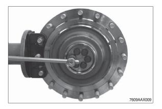
I Press planetary carrier with a two-armed puller out of the profile of the output shaft.
