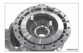
(9) Align disk package centrally and radially.
