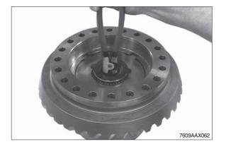
④ Remove spider shafts and axle bevel gears (see figure) out of the differential housing.
