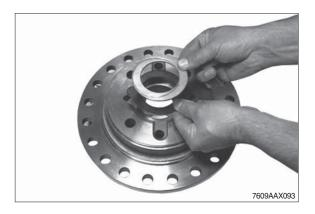
⑨ Mount two adjusting screws and insert the housing cover until contact with the differential housing is obtained.
