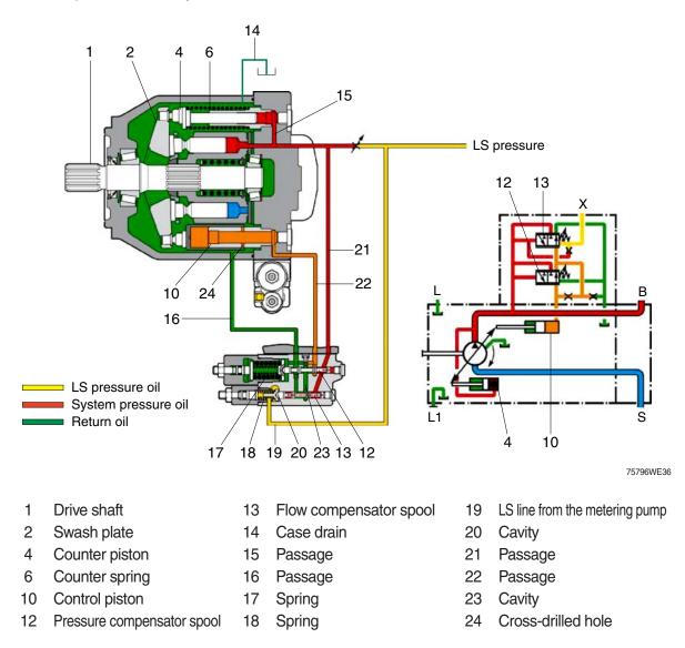
Low pressure standby constitutes the following condition: a running engine and inactive steering and loader. There are no flow demands on the pump or pressure demands on the pump. Therefore, there is no LS pressure in line (19).
