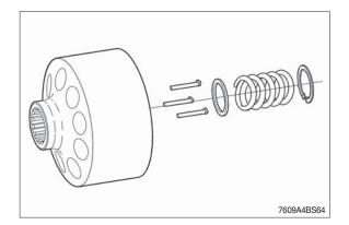
(7) Pre-tension the spring using a suitable device.
