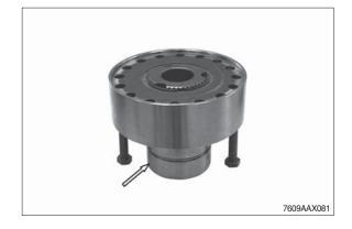
(6) Position the premounted differential with the lifting device onto the housing cover and preliminarily fix with hexagon screws.
