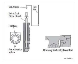
(3) Apply a light coating of clean hydraulic fluid to the spool and slide itinto the sleeve along with the ball checks if applicable.
