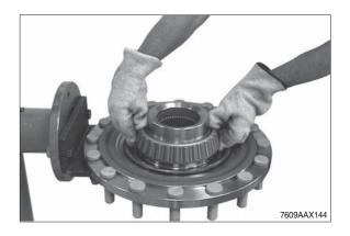
③ Wet O-ring of slide ring seal and locating hole with spirit.
