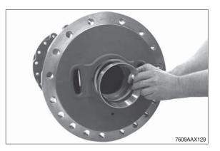
(9) Mount two locating pins and bring the axle housing into contact position with the axle drive housing by means of the lifting device.
