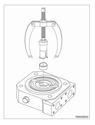
(6) Disassemble the taper roller bearing (near by port plate).Remove the adjustment shim.
