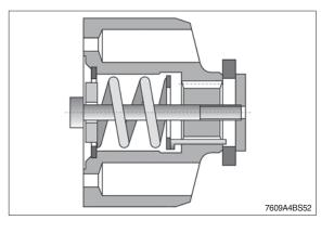
(16) Remove circlip. Remove spring and pressure pins.
