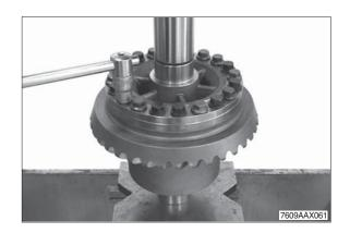
③ Lift the axle bevel gear with pressure ring, disk package and thrust washers out of the differential housing.
