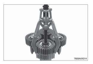
(4) Lift the end plate out of the brake housing.
