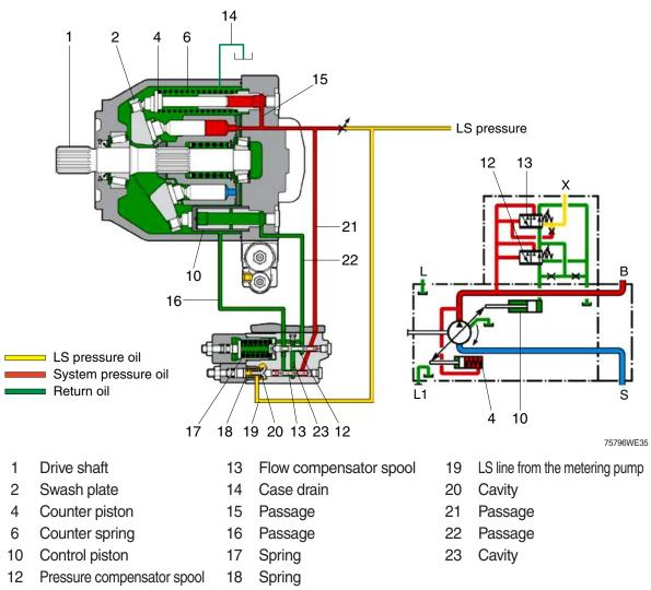
Upstroking of the pump occurs as flow demand from loader and steering system.
