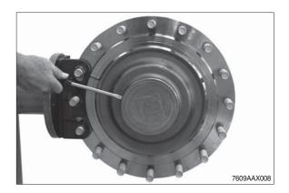
8 Loosen locking screws and remove the releasing cover.
