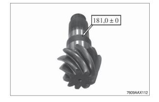
③ Determine dimension III (bearing width).
