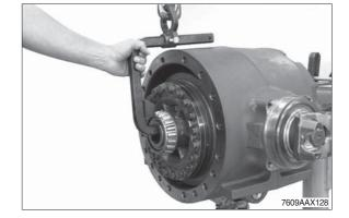
(B) Insert the determined shim (e.g. s = 1.1 mm) into the hole of the axle housing and adjust the bearing outer ring (see arrow) until contact is obtained.
