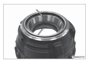
⑦ Clean the annular groove of the brake
