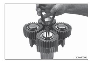
13 Pull off planetary gear.
