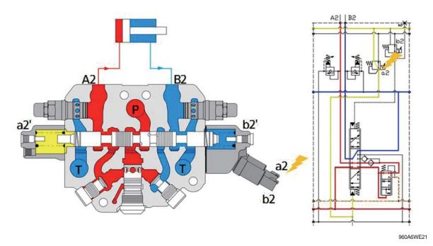
When the pilot pressure from EPPR valve (a2) is led to the port a2', the oil from the pump flows to the bucket cylinder (LC) port A2 and oil from the bucket cylinder (SC) flows into the tank through the bucket cylinder (sc) port B2.
