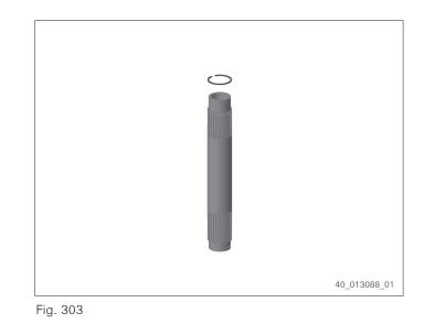
8. Insert turbine shaft in the input shaft until the snap ring audibly engages.
