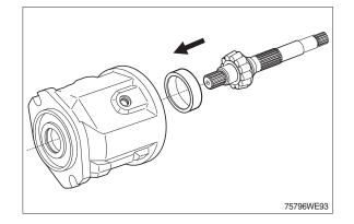
(3) Fit pressure pins using an assembly aid.
