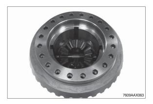
5 Remove the second axle bevel gear.
