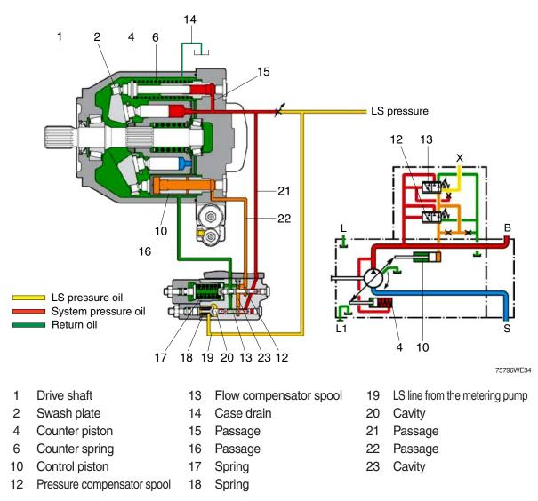
The decreased flow demand causes a LS pressure in line (19). The LS pressure in line (19) combines with the force of spring (18) in cavity (20).
