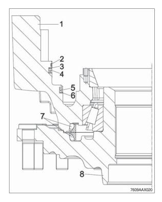
① Lift the brake housing from the output shaft by means of the lifting device.
