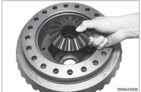
9 Press crown wheel from the differential carrier.
