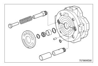
(5) Remove the rotary group in a horizontal position.
