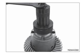
② Preload the differential by means of the press, loosen locking screws and housing cover.
