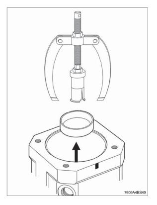
(13) Disassemble circlip and shaft seal.
