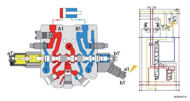
When the pilot pressure from EPPR valve (a1) is led to the port a1', the oil from the pump flows to the boom cylinder (LC) port A1 and oil from the boom cylinder (SC) flows into the tank through the boom cylinder (SC) port B1.
