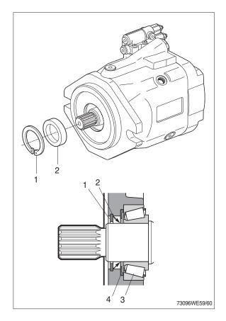
(1) Protect the drive shaft.Wrap the drive shaft with tape.Remove the retaining ring.Remove shaft seal to front.
