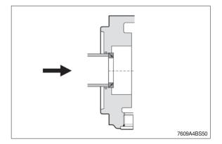
(14) Remove shaft seal and shim.
