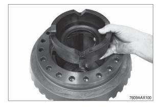
(5) Insert the axle bevel gear until contact is obtained and install the inner disks with the teeth.
