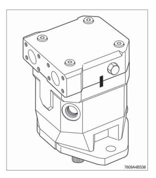
(2) Remove the port plate fixing bolts crosswise.
