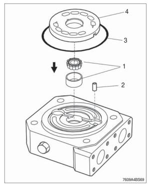
(11) Fit control plate. Assembly aid : Grease
