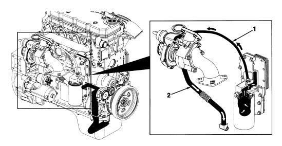
(1) Lubrication for the turbocharger
