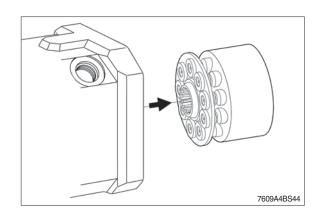
(8) Remove the drive shaft to rear side.
