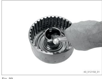
Pull off idler gear from shaft with 5870.300.024 [Disassembly device] and 5870.300.033 [Extractor].
