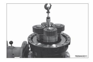
Pull the tapered roller bearing from the planetary carrier.
