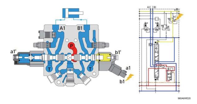
When the pilot pressure from EPPR valve (b1) is led to the port b1' to maximal pressure, the spool is in the forth position. The pump is in low pressure stand-by while port A1 and B1 are connected to tank.
