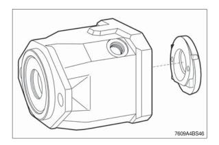
(10) Loosen the swash plate with a slide hammer (a small hook - diameter 6 mm catches the end of the swash plate at the bottom).
