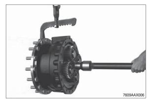
6 Fix output to assembly truck.
