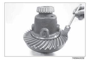
② Insert preassembled differential.
