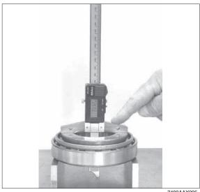
④ Undercool bearing outer ring (see arrow) and bring it into contact position in the inner bearing hole /pinion bearing by means of the fixture.
