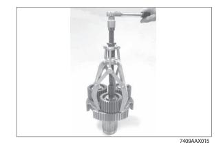
10 Pull bearing inner ring off the planetary carrier.
