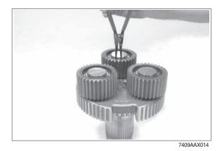
9 Pull off planetary gear.
