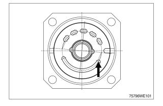
(10) Fit connection plate and control valve.
