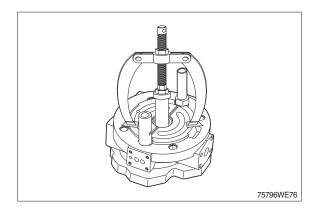
(13) Disassemble the guide of control piston (Mounting position: pilot valve side).
