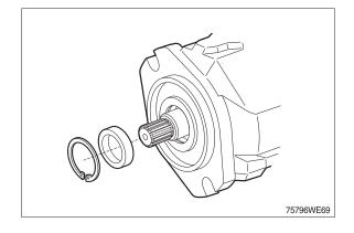
(8) Remove the drive shaft through rear side.
