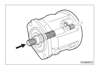
(9) Pre-tension the spring (1) using a suitable device.Remove circlip (2).Remove spring (1) and pressure pins (3).
