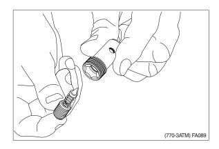
② Screw the adjustment screw so far in that the 10 mm hexagon key fully engages.
