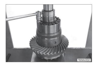
④ Preload the housing cover/compression spring by means of the press and disengage the retaining ring.
