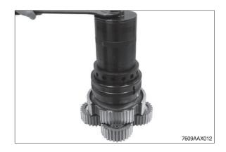
Disengage retaining ring.
