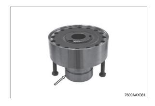
(f) Position the premounted differential with the lifting device onto the housing cover and preliminarily fix with hexagon screws.
