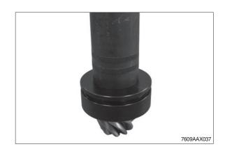
(9) If necessary, force both bearing outer rings out of the axle drive housing.
