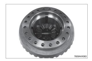
⑤ Remove the second axle bevel gear.
