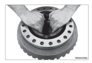
Press crown wheel from the differential carrier.
