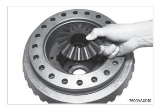
Press crown wheel from the differential carrier.
