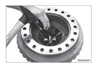
Pull the differential axle (long) and remove the releasing spider gears with thrust washers from the differential housing.
