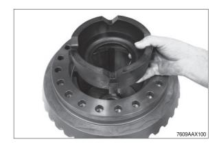
⑤ Insert the axle bevel gear until contact is obtained and install the inner disks with the teeth.
