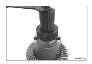
② Preload the differential by means of the press, loosen locking screws and housing cover.
