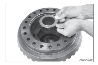
$\ensuremath{\mathfrak{I}}$  Insert axle bevel gear.
