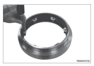
Insert the piston into the brake housing and carefully install with the fixing device until contact is obtained.
