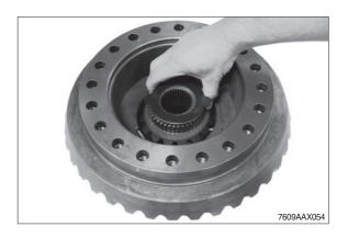
$\ensuremath{\mbox{\Large 5}}$  Force out both slotted pins.
