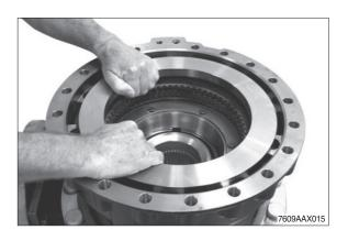
(5) Lift the disk package out of the brake housing.
