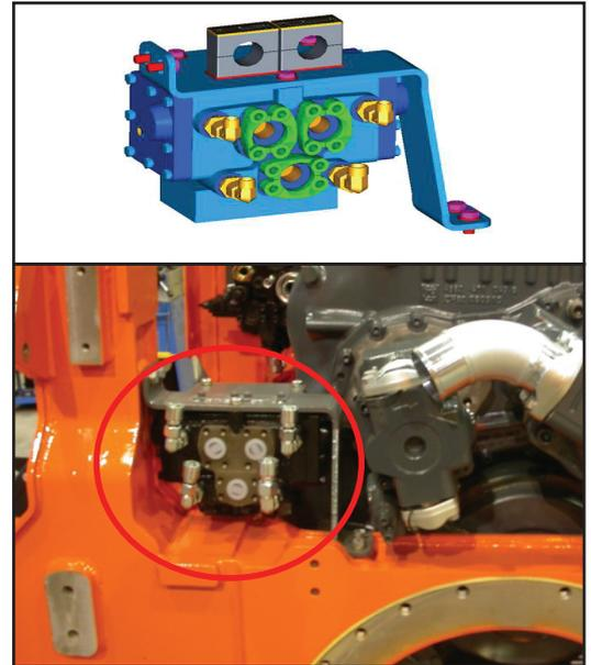
The Steering Valve is located on the front wagon, left-rear.
