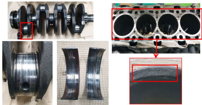
< Excessive wear of moving parts >
