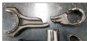
< Connecting rod broken >
