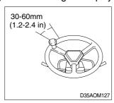
If the steering wheel play is over  $30\sim60\text{mm}$  (1.2-2.4in), check or repair it.
