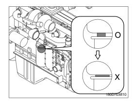
(8) Clean and inspect the oil drain plug threads and the seal surface. If any damage is found, the oil drain plug must be replaced. Install and tighten the oil drain plug.
