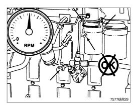
④ For faster air purge, small amounts of air can be bled from the fuel injection pump by operating the hand primer located on the fuel transfer pump or by cranking the engine.
