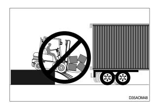
▲ The impact of moving in and out of a trailer may cause the trailer to creep or move.
