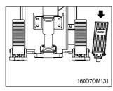
With the parking brake released and the direction control in FORWARD or REVERSE, put your foot on the accelerator pedal and push down smoothly until the truck is moving at the desired speed.
