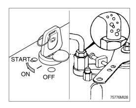
③ Since the fuel transfer pump provides positive pressure through the fuel filter and supply line to the fuel injection pump, loose connections or defective seals can show as a fuel leak, not as an air leak.
