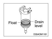
(2) When the float of separator meets the red line(drain level), drain water.
