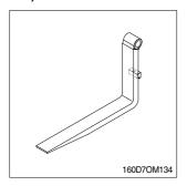
The load forks are adjustable on the hanger, carriage. Forks should be spaced as far apart as the load will allow. Both forks should always be the same distance from the center of the fork carriage. To adjust the forks, raise the carriage slightly. Tilt the mast fully forward to reduce friction and make the fork slide easier.
