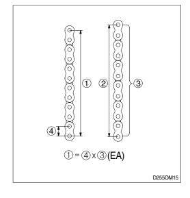
All chains must be replaced if any link has wear of 3% or more, or if any of the damaged conditions notes above are found during inspection. Order replacement chains from your HYUNDAI dealer. Replace all chains as a set. Do not remove factory lubrication or paint new chains. Replace anchor pins and worn or broken anchors when installing new chains. Adjust tension on new chains. Lubricate chains when they are installed on the mast.
