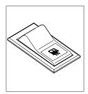
(1) This switch is used for the fuel heater of the pre-heater assy.
