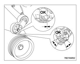
(4) Inspect the tensioner for evidence of the pivoting tensioner arm contacting the stationary circular base. If there is evidence of these two areas touching, the pivot tube bushing has failed and the tensioner must be replaced.
