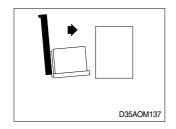
① Approach slowly and align the lift truck and load squarely with the stack.
