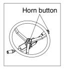
(1) If you press the button on the top of the multifunction switch and the center of the steering wheel, the horn will sound.
