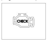
① This lamp lights ON during a nonfatal engine system error. The engine can still be run, but the fault should be corrected as soon as possible.
