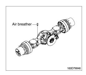
(3) Remove the plug and check the oil amount. If the oil level is at the hole of the plug, it is normal.
