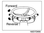
Push the direction control lever forward, center it, or pull it back for FORWARD, NEUTRAL, or REVERSE, respectively. Traction is disabled in NEUTRAL.
