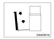
⑦ Check your travel path, then carefully back away until the forks are clear of the stack. Stop and lower the forks to the travel position[150~200mm(6~8in) above the ground], then tilt back for travel.
