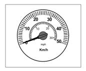
① The speed meter displays the speed of truck in mph and km/h.
