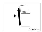
③ Move forward slowly until the load almost touches the stack. The leading edge and sides of the load pallet should line up exactly with the near edge and side of the load or rack on which you are stacking.
