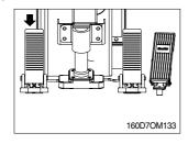
Use the inching pedal and the accelerator pedal in combination to vary lift and travel speeds independently. The further you depress the inching pedal, the more the driving clutch slips, reducing travel motion. With the inching pedal fully depressed, the brakes fully engage. You operate the inching pedal with your left foot for precise control of travel speed, while you operate the accelerator pedal together with the lift control to vary lift speed.
