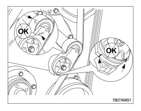
(3) Check that the bottom tensioner arm stop is in contact with the bottom tensioner arm stop boss on the tensioner body. If these two are not touching, the tensioner must be replaced.
