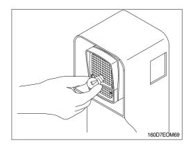
▲ After checking that the fuse is not blown and that there is no disconnection in the wiring harness, replace the lamp bulb.
