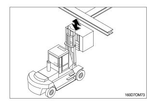
▲ Watch overhead clearance: Moving into overhead structures can tip a truck over, or spill a load.
