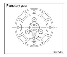
(5) After draining, put the drain plug of planetary gear in parallel to the ground.
