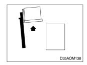
② Raise the load as the lift truck nears the stack.
