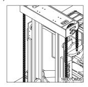
Raise forks 10 to 15cm(4 to 6in) from ground. Push with a rod to check that both chains have approximately same amount of slack.
