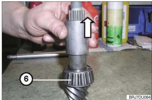
**(6) Removal of thread protective shield and radial sealing ring**
