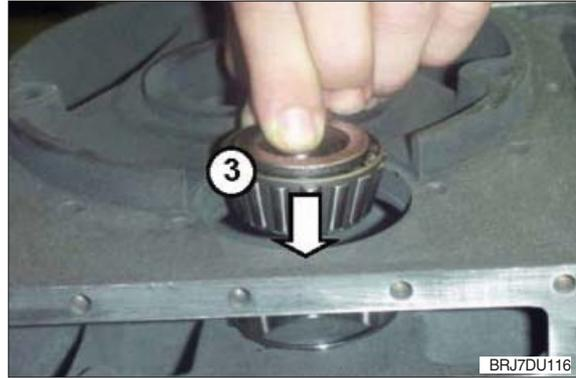
**(1) Installation of grooved ball bearing for drive pinion**
