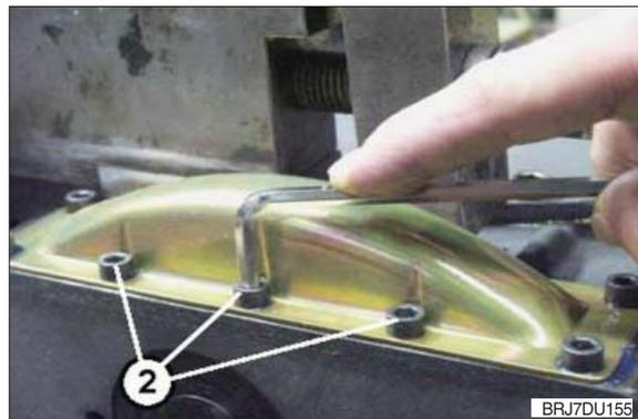
**▲ Do not yet tighten the cap screws with the corresponding tightening torque.**
