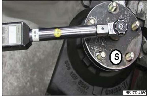
Bearing preload is adjusted correctly when a bearing friction torque of 8.0 ~ 22 Nm is obtained at the wheel shaft.
