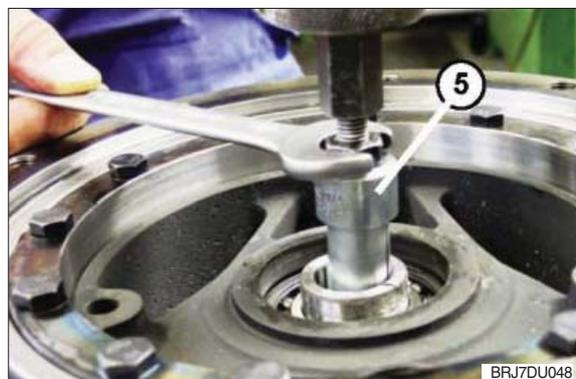
(5) Handle the extracting fixture "S" as shown on the right. Move the handle on the bar upwards strongly several times until the drive pinion is loosened from the bearing seat completely.
