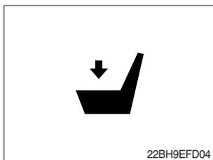
This LED lights when the operator is not on the seat.
