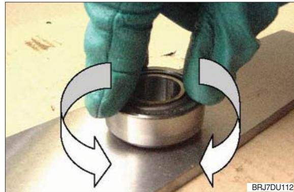
③ Measuring of bearing slack H.
