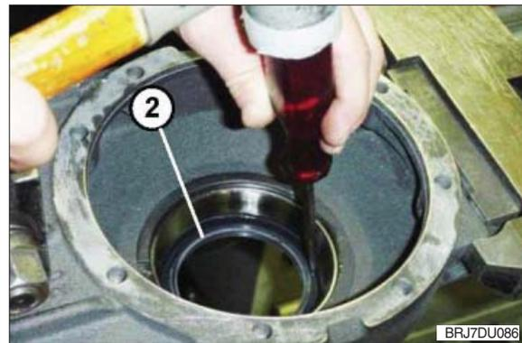
**(7) Disassembly of bearings**
