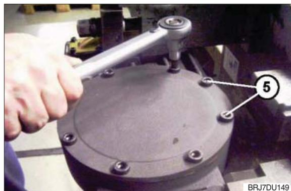
**(5) Checking of bearing friction torque on wheel shaft**
