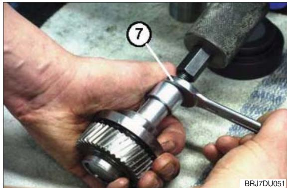
(8) Pull of the grooved ball bearing (item 8) by means of a puller or a parting tool over the bearing seat of the drive pinion and dispose it of according to chapter 6.
