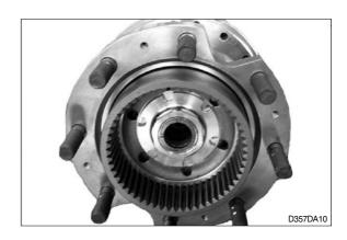
(11)Remove bearing cup from the wheel hub by using jig and hammer. Shaft seal will be damaged.
