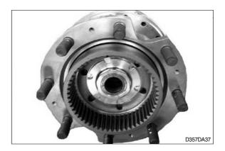
(3) Insert shim, fix the torque plate and ring gear with snap ring and assemble them to the axle tube.
