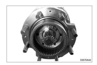
(6) Assemble internal components of planetary carrier in the reverse order to disassembly.
