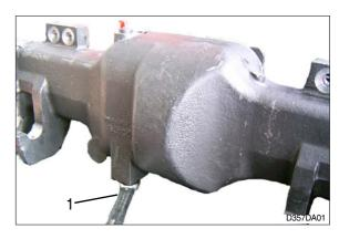
(2) Loosen 4 socket head bolts(2) and a plug(3) from the housing of planetary.
