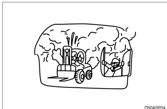
▲ Be particularly careful when removing the radiator cap and the hydraulic oil tank filler cap, if this is done immediately after using the machine, there is a danger that boiled oil may spurt out.
