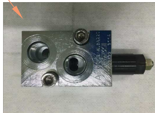
② Counter balance valve block
