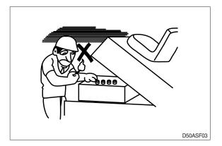
• Exhaust gas is dangerous. Provide adequate ventilation when working a closed space.
