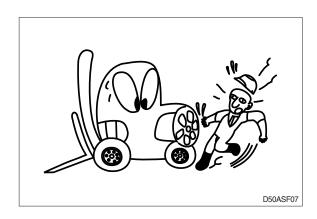
When inspecting running parts or near such parts, always stop the machine first.
