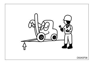
Immediately remove any oil or grease on the floor of the operator's compartment, or on the handrail. It is very dangerous if someone slips while on the machine.
