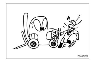
When inspecting running parts or near such parts, always stop the machine first.
