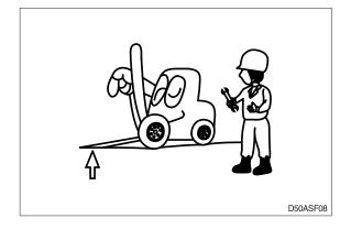
Immediately remove any oil or grease on the floor of the operator's compartment, or on the handrail. It is very dangerous if someone slips while on the machine.
