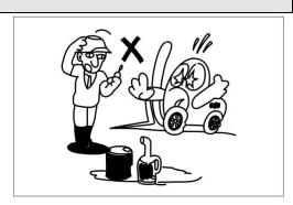
Wear well-fitting helmet, safety shoes and working clothes. When drilling, grinding or hammering, always wear protective goggles. Always wear safety clothes properly so that they do not catch on protruding parts of truck. Do not wear oily clothes.
