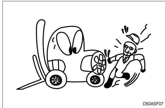
When inspecting running parts or near such parts, always stop the machine first. Before checking or servicing accumulator or piping, depress brake pedal repeatedly to release pressure.
