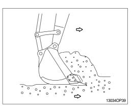
4) Set the tracks parallel to the line of the ditch to be excavated when digging ditch. Do not swing while digging.
