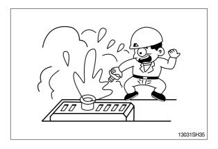
Do not work below the machine. Be sure to work with proper safety supports. Do not depend on the hydraulic cylinders to hold
