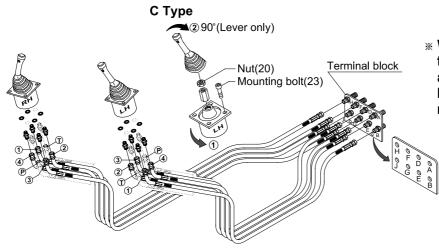
Whenever a change is made to the machine control puttern also exchange the pattern label in the cab to match the new pattern.
