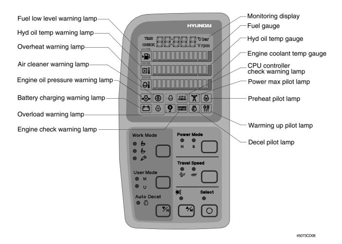
\* The warning lamp lights ON and the buzzer sounds when the machine has a problem.
