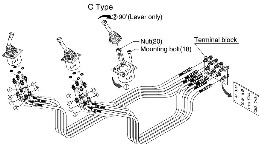
\* Whenever a change is made to the machine control pattern also exchange the pattern label in the cab to match the new pattern.
