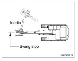
Do not use the dropping force of the work equipment for digging. The machine can be damaged by the impact.
