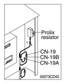
(1) This resistor is used to continuous working in case of malfunction of the CPU controller.
