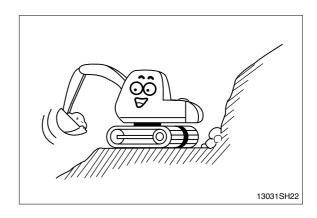
The swing on the slope can be danger of rolling over.
