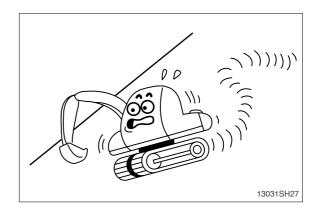
The engine angularity limits are 35 degree.
