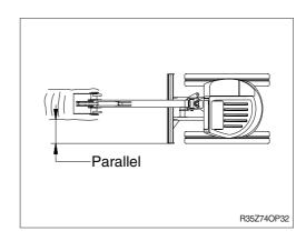
5) Dig slowly with keeping the angle of boom and arm, 90-110 degree when maximum digging force is required.
