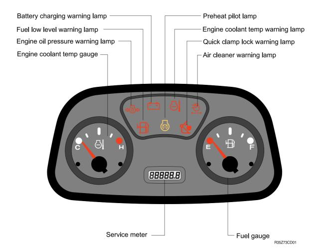
\* When the quick clamp switch turn ON, the buzzer sound and the quick clamp warning lamp lights ON.
