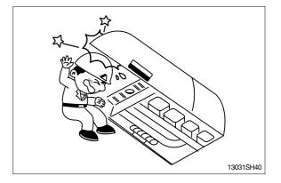
The antislip protection should be replaced if they have become worn or have been printed over. Be sure to free of oil, water and grease etc.
