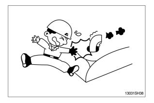
Do not open the engine hood and covers while the engine is running.
