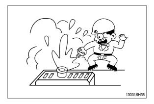
Do not work below the machine. Be sure to work with proper safety supports. Do not depend on the hydraulic cylinders to hold up the equipment and attachment.
