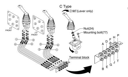
Whenever a change is made to the machine control pattern also exchange the pattern label in the cab to match the new pattern.
