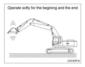
3) The digging resistance and wearing of tooth can be reduced by putting the end of bucket tooth to the digging direction.
