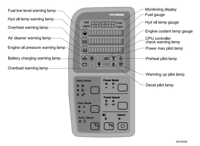
\* The warning lamp lights ON and the buzzer sounds when the machine has a problem. In this case, press the buzzer stop switch and buzzer stop, but the warning lamp lights until the problem is cleared.
