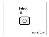
This switch is used to select the monitor display function.
