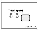
This switch is to control the travel speed which is changed to high speed(Rabbit mark) by pressing the switch and low speed(Turtle mark) by pressing it again.
