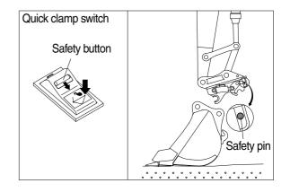
(3) Aligning the arm and bucket, insert static hook of quick clamp to the bucket pin.
