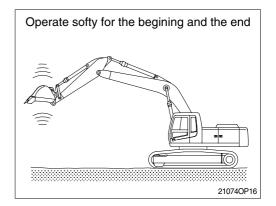
The digging resistance and wearing of tooth can be reduced by putting the end of bucket tooth to the digging direction.
