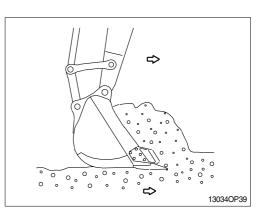
Set the tracks parallel to the line of the ditch to be excavated when digging ditch. Do not swing while digging.
