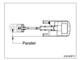
Dig slowly with keeping the angle of boom and arm, 90-110 degree when maximum digging force is required.
