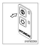
(1) This switch makes the system and the LED simultaneously ON or OFF.
