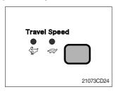
① This switch is to control the travel speed which is changed to high speed(Rabbit mark) by pressing the switch and low speed(Turtle mark) by pressing again.
