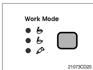
① This switch is to select the machine operation mode, which shifts from general operation mode to heavy operation mode and breaker mode in a raw by pressing the switch.
