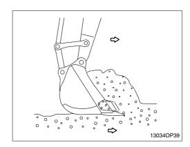
Set the tracks parallel to the line of the ditch to be excavated when digging ditch. Do not swing while digging.
