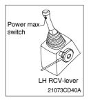
(1) This switch activate power max function.When this switch is kept pressed, hydraulic power of work equipment
