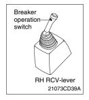
(1) On pressing this switch, the breaker operates only when the breaker selection switch on the switch panel is selected.
