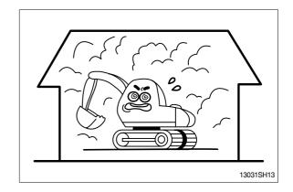
Check the locations of underground gas pipes or water line and secure the safety before operation.
