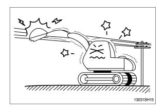
If the machine touches the electric power lines, keep sitting on the operator's seat and make sure the personnel on the ground not to touch the machine until turning off the electric current. Jump off the machine do not contact the machine when you need to get off.
