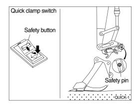
(3) Aligning the arm and bucket, insert static hook of quick clamp to the bucket pin.
