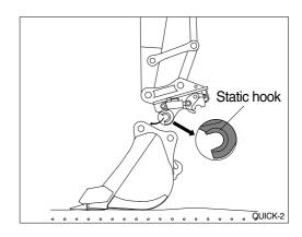
(4) Operate RCV lever to bucket-in position. Then, the moving hook is coupled with the bucket link pin.
