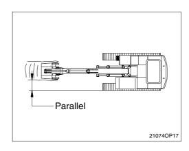
5) Dig slowly with keeping the angle of boom and arm, 90-110 degree when maximum digging force is required.
