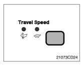
① This switch is to control the travel speed which is changed to high speed(Rabbit mark) by pressing the switch and low speed(Turtle mark) by pressing again.
