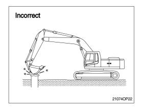
10) Do not use the bucket to crack hard objects like concrete or rocks.
