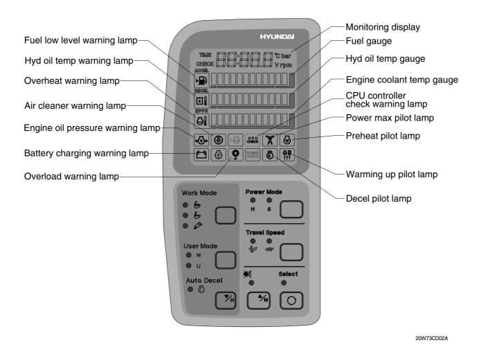
\* The warming lamp lights ON and the buzzer sounds when the machine has a problem. In this case, press the buzzer stop switch and buzzer stop, but the warming lamp lights until the problem is cleared.
